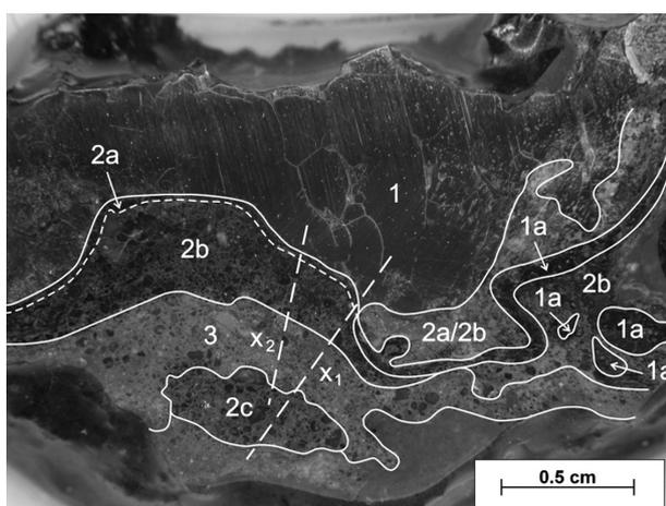
**Fig. 2.** SEM picture of the 970-g meteorite, with macroscopic interpretation of its coating structure. A portion of this photograph was published in Fedorowicz & Stankowski (2016).
