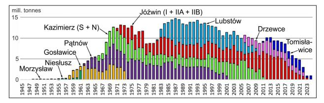
Fig. 4. Lignite mining in the Konin Lignite Mine (KLM) in the years 1945–2024 (based on mining data). Note the years and volume of lignite exploitation in individual opencasts.
