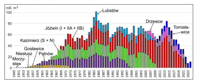
Fig. 5. Overburden removal in the Konin Lignite Mine (KLM) in the years 1945–2024 (based on mining data). Note the years and volume of overburden removal in individual opencasts.
